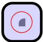
**Corner:** Our standard hinge corner is 1/4" Radius Corner. Other corner specifications are Square Corner and 5/8" Radius Corner. All hinges are mortised into the jamb and door.
