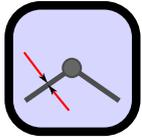
**Thickness:** The thickness of the leaves are measured in Imperial Gauge or Millimeters. But often sold by generic names like "residential" (thin) or "heavy duty" (thicker). Residential hinges are typically 2mm-2.5mm and Heavy Duty hinges are typically 3.0mm-3.5mm in thickness.
