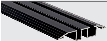
**THE COMMERCIAL SILL** IS ADA COMPLIANT AND IS AN OPTION WHEN INTERIOR AND EXTERIOR FLOOR LEVELS ARE THE SAME AND A MAXIMUM SILL HEIGHT FROM FINISH FLOOR OF 1/2" IS REQUIRED. ADEQUATE OVERHANGS ARE RECOMMENDED TO REDUCE THE RISK OF WATER INFILTRATION.
