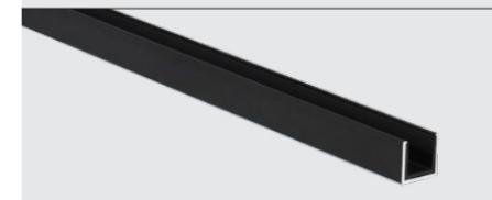
**THE GUIDE CHANNEL SILL** OPTION IS RECOMMENDED FOR INTERIOR APPLICATIONS WHEN FLOOR LEVELS ARE THE SAME. IT IS NOT SUITABLE FOR EXTERIOR USE UNLESS AIR INFILTRATION IS ACCEPTABLE OR THERE IS NO RISK OF WATER INFILTRATION.
